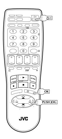
The Auto Set Up function simplifies installation by guiding you through the procedures of setting the clock and tuner channels — simply follow the on-screen menus that appear when the  $\theta/1$  button is first pressed to power on the recorder after you plug the mains power cord into a mains outlet.
