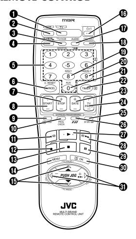
Buttons with a small dot on the left side of the name can also be used to operate your TV  $\square Pg$  93.
